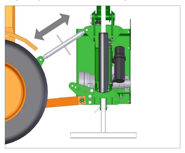
5. Attach stabiliser bars to the nearest available hole, ensure both bars are located in the same hole in both sides. Before fully tightening the bolts, lower the linkage to allow the weight of the machine to be taken by the stabiliser bars, then fully tighten
