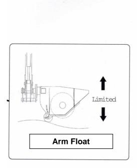
This is only to be used in verge mowing set up, it will reduce weight on the rear roller allowing head to move more easily, following small changes in ground contours in a forward motion, with the aid of a pre-charged gas accumulator.
