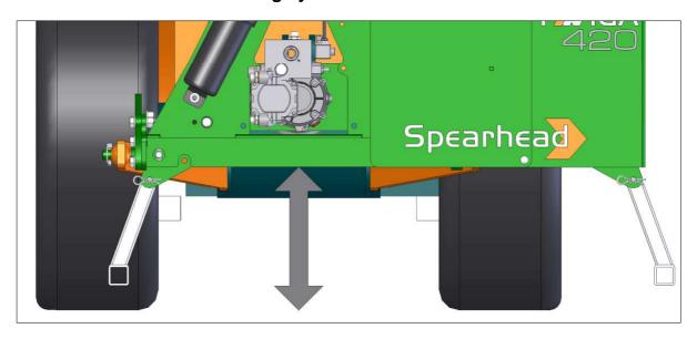
4. Adjust the top link so that the machine sits vertically
