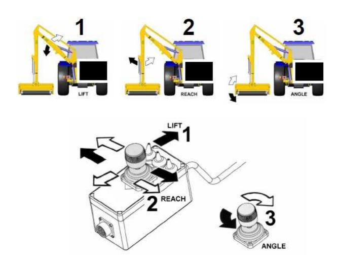
Before commencing work it is advisable to find an unobstructed level site and operate the machine through its entire range of movements to familiarise yourself with the controls and the machines response to them. This is a wise precaution for all operators and a must for the inexperienced.
