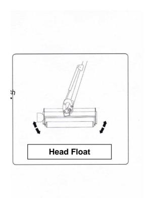
This option allows the flail head to follow contours of the ground without having to constantly control the angle of the head.
