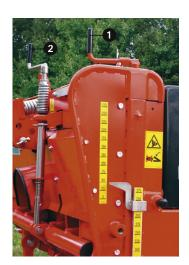
Achieve different spiking intensities by adjusting the entry angle of the tines.
